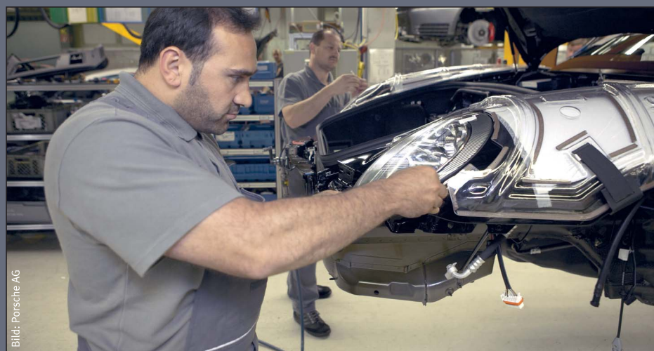
Installation of the main headlights: Part of the Porsche philosophy is that certain parts such as the left headlight always get the same UL-ID (Usage Location Identification). In this way errors can be avoided both in development and in assembly plus service.
